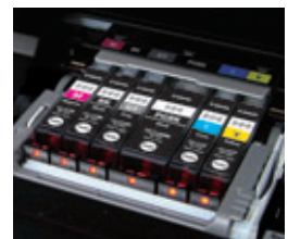
LED blinks when ink is running out
