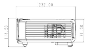
Lens center: 96 mm from the left side ('front" is the side where lens is attached.)
