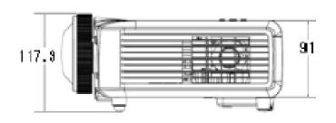
Lens center: 96 mm from the left side ('front" is the side where lens is attached.)
